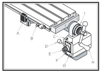
Figure 22. Power feed system components.
